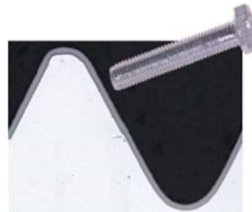
Figure 2. Micrograph showing cross section of Tantaline treated Fastener. Original profile is preserved.
